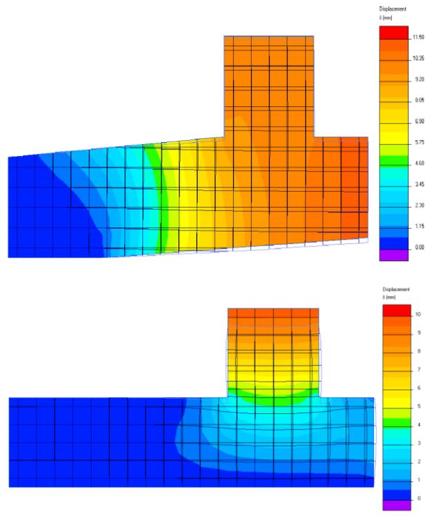
**Fig. 6.** Distribution of total displacements in the adaptive tire in the contact area with the rolling track
