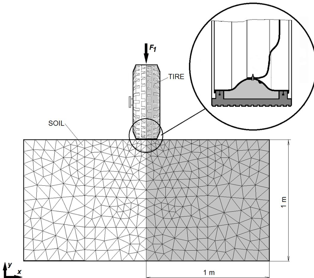
**Fig. 4.** Analysis model for the adaptive tire-soil interaction
