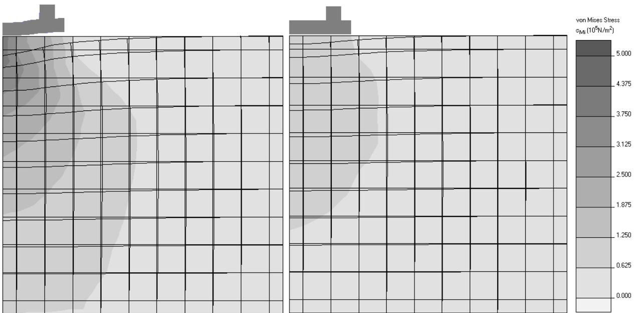
**Fig. 7.** Comparative analysis of distribution of equivalent stresses in agricultural soil for the two situations of adaptive tire operation
