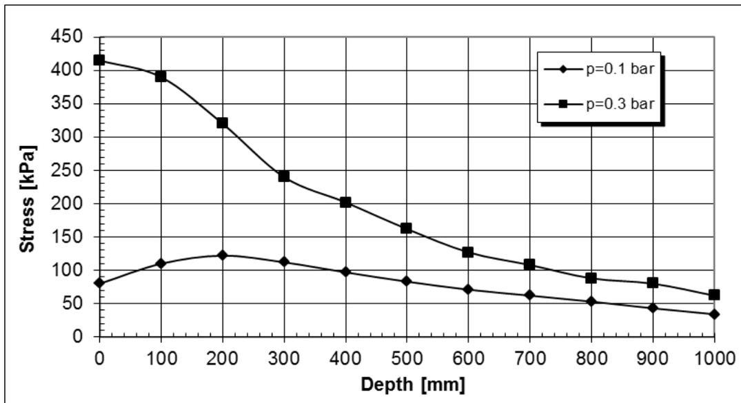
**Fig. 8.** Graphical variation of equivalent stresses in agricultural soil with depth, for the two situations of adaptive tire operation
